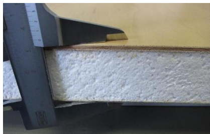
Example sandwich: aluminum - insulation - plywood
