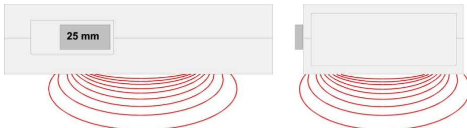
Side view: measuring field and penetration depth for switch setting "25 mm"
