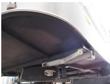
Caravan floor: massive flake board, little protected
