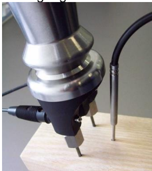
Reciprocating piston electrode GHE 38 with temperature-probe GTF 38
