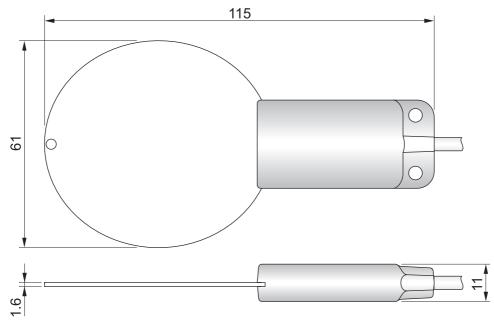
Fig. 1: dimensions (mm)
